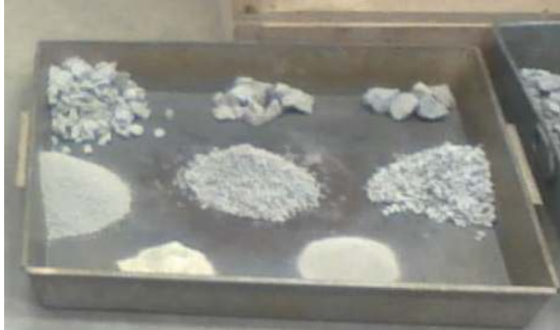
Figure 3.36. Piles of individual particle sizes matching the gradation of interface samples obtained in November 2010, and placed in three foot by three foot metal pans.
