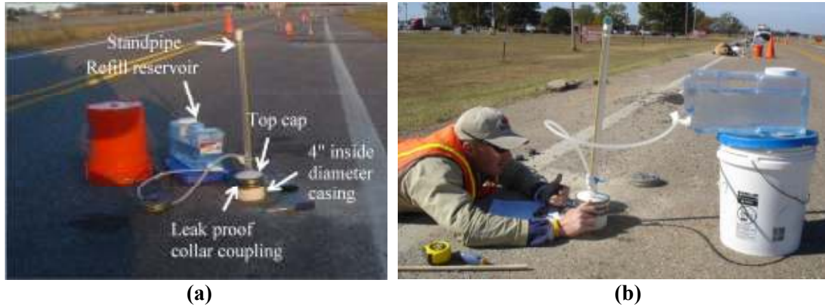
Figure 3.20. a) Two stage borehole setup prior to testing and b) ongoing two stage borehole test.
