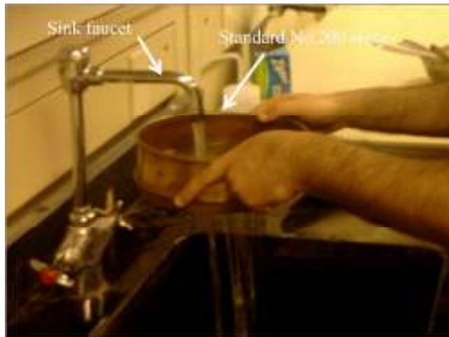
Figure 3.26. Wash sieving of subgrade sample using a standard No. 200 sieve.
