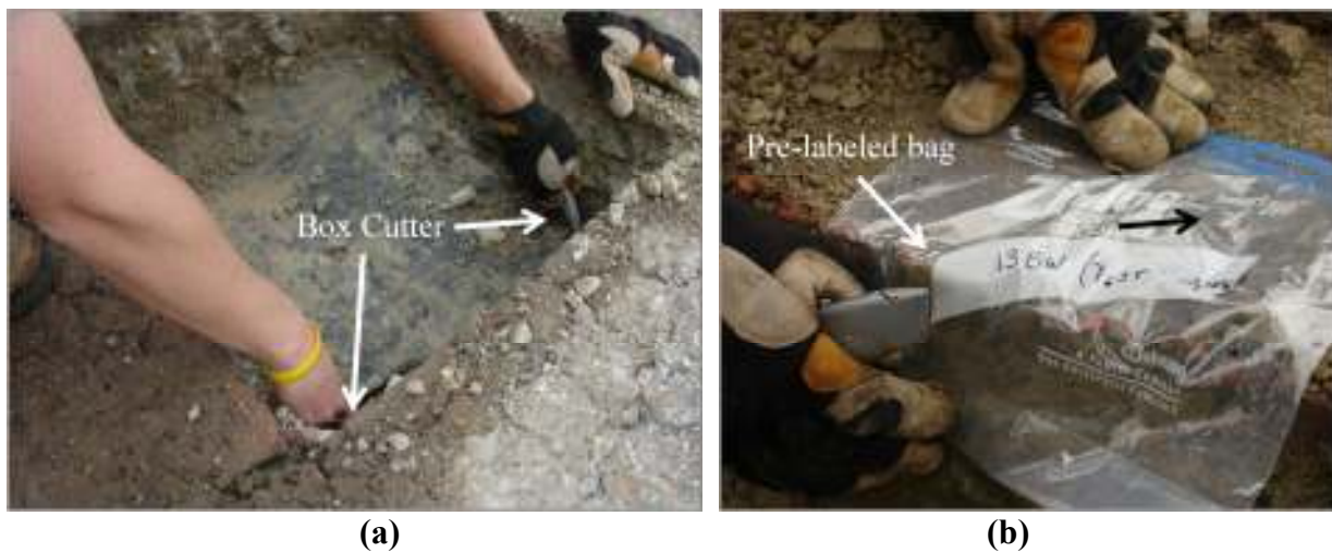
Figure 3.13. Geosynthetic sample a) removal using a box cutter and b) pre-labeled bag ready for placement.
