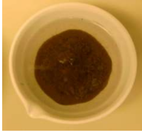
Figure 3.25. Subgrade sample being soaked in water prior to wash sieving.
