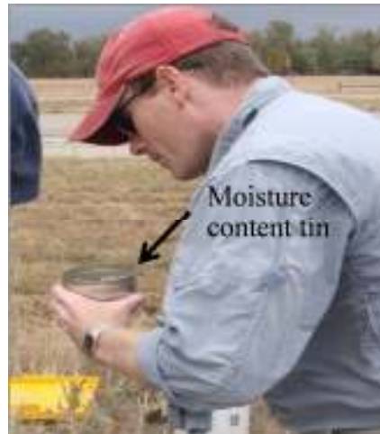
Figure 3.12. Base course moisture content sample.
